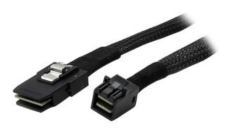
This internal mini-SAS cable provides a cost-saving solution for connecting a SAS or SATA adapter to a SAS or SATA backplane that has an SFF-8087 connection.
